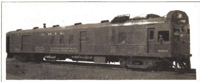
The Erie Is Spending Millions on Modern Equipment to Help the Unemployed and at the Same Time to Buy at Bargain Prices. Above We See a New Type of Gasoline-Electric Combination Mail-Express Car
