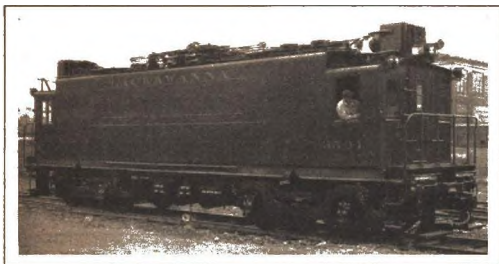
One of the Lackawanna's Two New "Three-Power" Locomotives, Uniquely Designed for Transfer and Switching Service. These Are the First of Their Kind Built to Operate at 3,000-Volt Direct Current from Overhead, Instead of Third-Rail Contact
